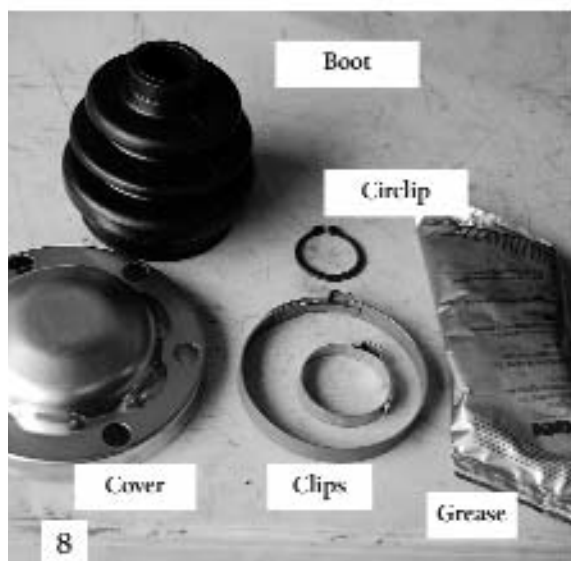
No. 6: A small clip secures the boot to the axle. Cut it off; a new one is in the kit.
