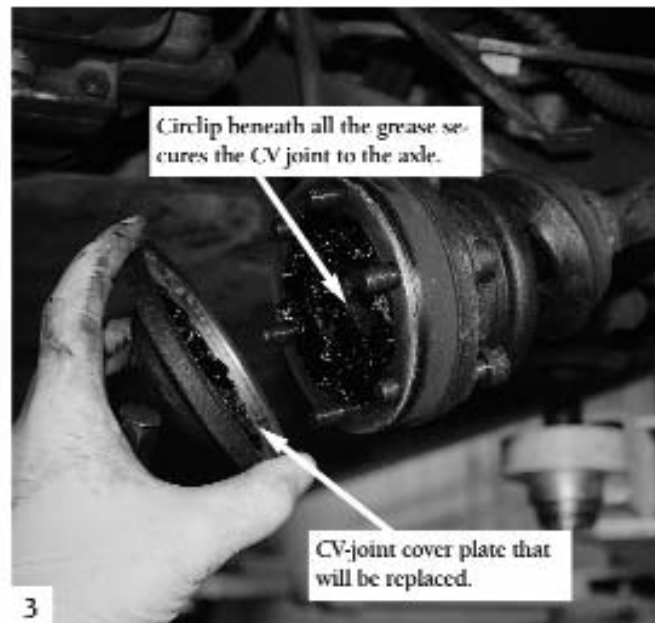
No. 3: With the joint separated from the transaxle, the cover should pop off. Leave the bolts in the joint. Beneath all that black grease is a circlip. Use circlip pliers to remove the circlip; a new one is included in the kit.
