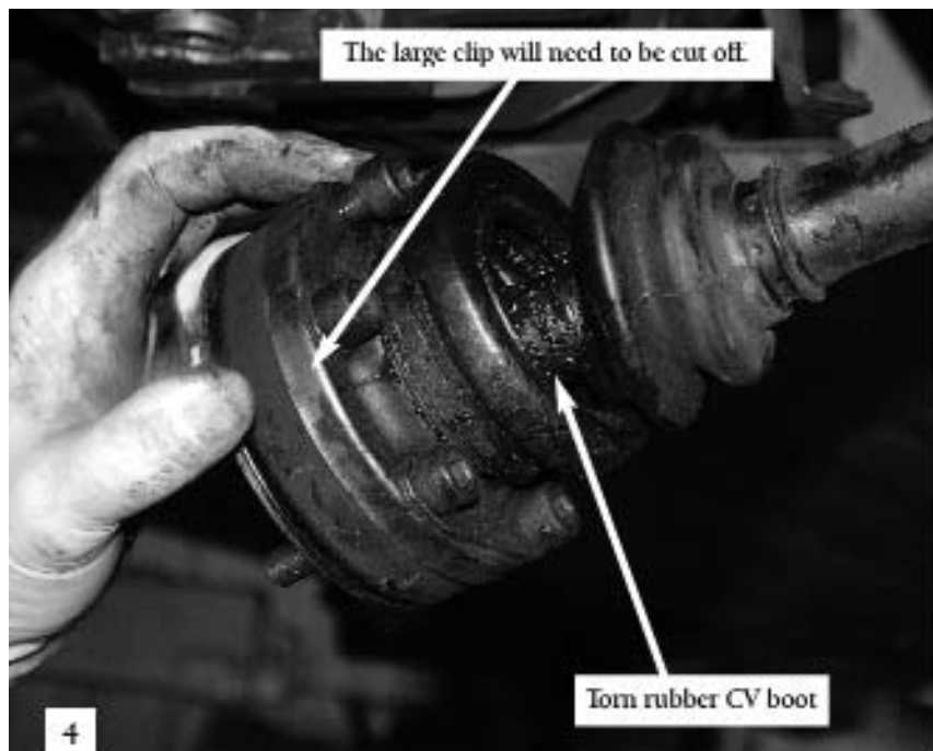
No. 4: Luckily, this torn boot was discovered and replaced before the CV joint was ruined.
