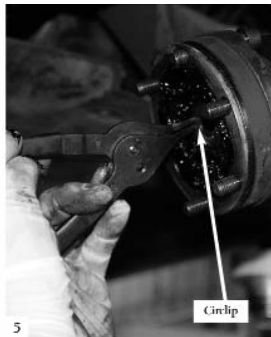
No. 5: Use circlip pliers to remove the circlip that secures the CV joint to the axle.
