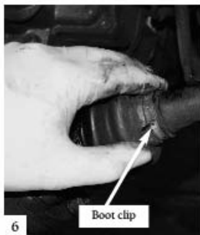
No. 4: Luckily, this torn boot was discovered and replaced before the CV joint was ruined.
