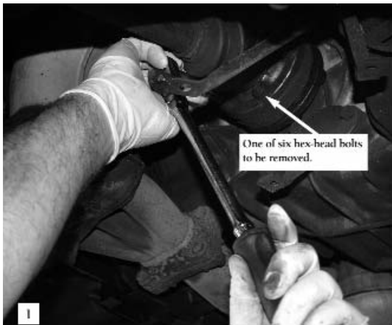
No. 1: Chapman loosens the six hex-head bolts first with a ratchet, then removes them with an air ratchet to save time. It's important to leave the car out of gear in order to rotate the axle to access all six bolts.
