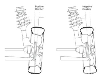
A proper racing suspension has geometry which gains negative camber as the body rolls. Modern Porsches with their MacPherson strut suspension have limited camber gain as the body rolls during a corner. Given this condition, plus the fact that some negative camber maximizes cornering
