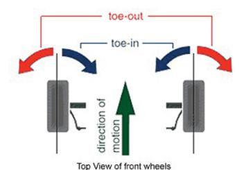
Toe settings affect tire wear, directional stability, and corner entry handling characteristics. Any toe causes the tires to scrub. Too much toe-in causes excess wear on the outside of the tire and too much toe-out wears the inboard edges. A little toe-in at the front wheels helps with straight line stability but the trade-off is some loss of turn-in ability. A little toe-
