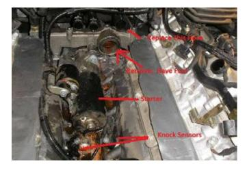
Once all the pieces are finally removed, you can reassemble with the new aluminum tubes. The large pipe is a 3 piece tube, so inserting it is easier than removal. Here the lower pipe is installed, along with the upper thermostat housing.
