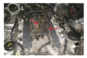
The lower pipe shown here is a little harder to remove. The pipe needs to be cut in order for it to be removed due to the assembly of the engine.
