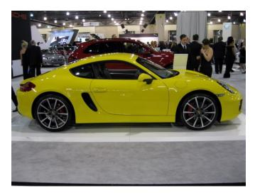
The most noticeable change from either side, are the new black side air intakes. Both intakes are functional and move more air into and around the engine compartment than before. I like this new look as it reminds me a little of a 911 Turbo.
