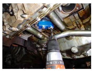
We now have a perfect hole in the cylinder head. All that is left in the hole are the threads of the old stud. With a small dental pick, you can peel out the old threads. Once you get the tip of the threads exposed, grab them with a pliers, and slowly pull downward, unwinding them out of the head.
