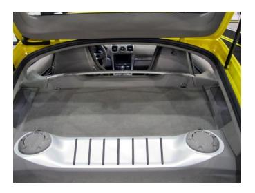
The deck above the engine compartment has a lip maybe three or four inches high all of the way across from one side to the other in order to prevent anything from sliding forward into the back of the seats. Because of this lip, it makes the storage area above the engine look bigger and more useful.
