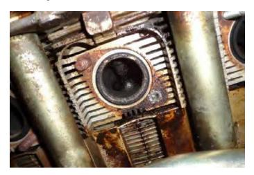
Here we have all that was left of the old rotten stud, a nice coil of threads. The result is that the original tapped threads remain in the cylinder head completely untouched. This is a very precise tool indeed.
