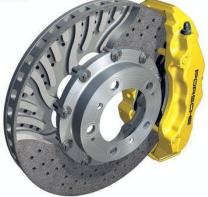
Like a competition-bred conventional system, the ceramic outer disc is mated to a steel inner "hat." PCCB brakes use specially developed six-piston calipers on the front and four-piston calipers on the rear.
