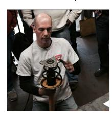
crew as why this was important, especially if you didn't want to repair your garage ceiling or visit an ER. Once compressed, the strut mount was removed via an impact wrench and a box wrench. The strut was than disassembled and reassembled with the spanking new yellow Bilstein.
