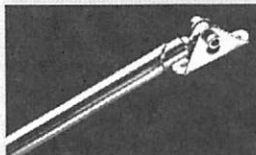
STRUT TOWER BRACES
