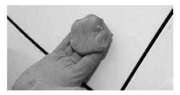
**Step 1:** Before starting the compounding process, Tim wipes down the car with a clay bar. Simply spray a section of paint with a quick detailing product, such as Prima's Glide, and then run the clay over the finish. The clay will grab contaminants from the surface.
