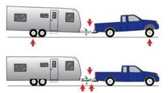
Every full-size pickup sold today is required by the vehicle's manufacturer to use a weight-distributing hitch to tow trailers weighing above a certain weight, and that weight limit for the majority of pickups is 5,000 pounds regardless of cargo. The owner's manual for Dan's Tundra requires a weight-distribution hitch if the gross trailer weight exceeds 5,000 lbs., and Dan's trailer was well over that weight.
