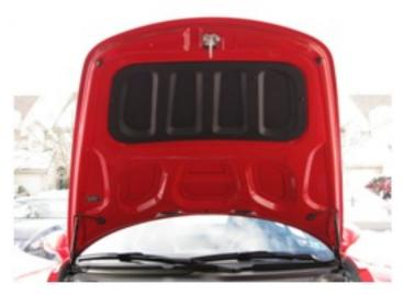
Here is the hood with the lid liner installed.
