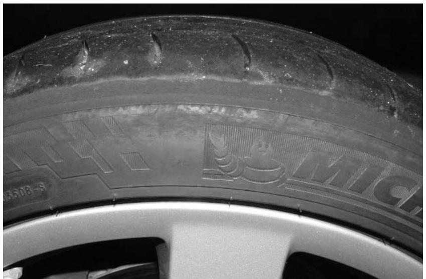
Michelin PS2 after several track days. Note absence of "Z" pattern and how much less the radial grooves wrap shoulder. This is evidence of roll-over.
