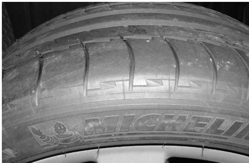
Almost new Michelin PS2, note "Z" pattern on shoulder and how radial grooves wrap shoulder.
