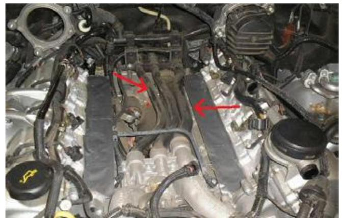
The lower pipe shown here is a little harder to remove. The pipe needs to be cut in order for it to be removed due to the assembly of the engine.
