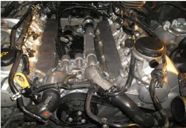
After that, you can install the upper aluminum pipes and button everything back up on top of the engine. There is also a coolant hose on the back of the engine that should be replaced at the same time. Another fun time, as the hose tends to seize itself to the hard line.
