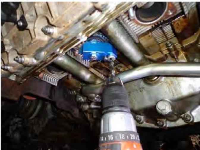
We now have a perfect hole in the cylinder head. All that is left in the hole are the threads of the old stud. With a small dental pick, you can peel out the old threads. Once you get the tip of the threads exposed, grab them with a pliers, and slowly pull downward, unwinding them out of the head.
