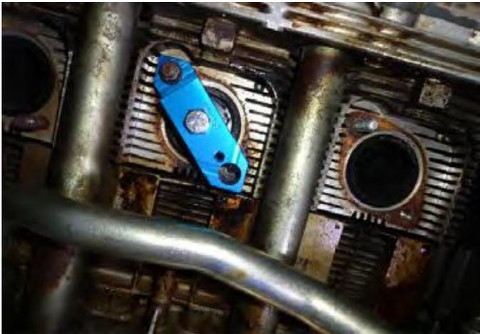
bushing and you can see up through the tool at the hole you have made in the stud.
