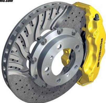
Like a competition-bred conventional system, the ceramic outer disc is mated to a steel inner "hat." PCCB brakes use specially developed six-piston calipers on the front and four-piston calipers on the rear.
