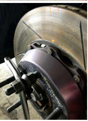
stud. Once complete, pop the wheels back on and torque the lug nuts to 90 – 95 ft/lbs. You now have studs. Being under stay at home orders, I was in no rush to get through this project, and it took me about two hours. If I were in a hurry I could probably have done it in half the time.
